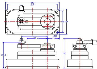
The Jefa 150 KgM direct drive type 1 is very compact with a length of 345 mm, a width of 164 mm and a height of 192 mm. As space is always a problem on sailing yachts, the direct drive unit can be mounted as close as 250 mm from the rudderstock even upside down.
