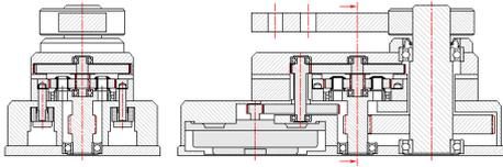
This assembly drawing shows a cross section of the direct drive type I. The drive can be separated in 5 main parts: The electric motor, the two step spur gearbox, the planetary gearbox, the electro-magnetic clutch and the final spur reduction gearbox. The Jefa direct drive has multiple advantages over existing integrated drive units. These advantages will be explained per section of the drive:
