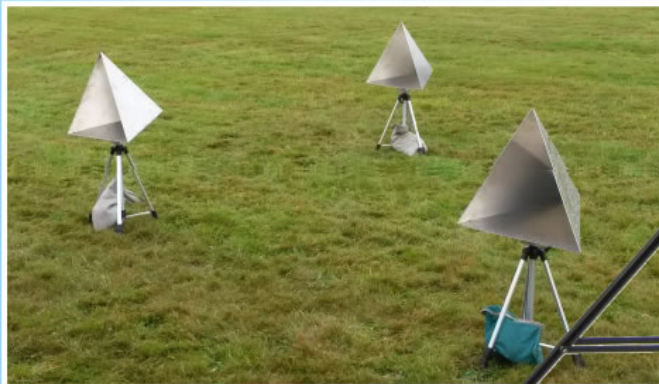
Three EMTH50 Reflectors being used to test response of helicopter radars at 6000 feet.
